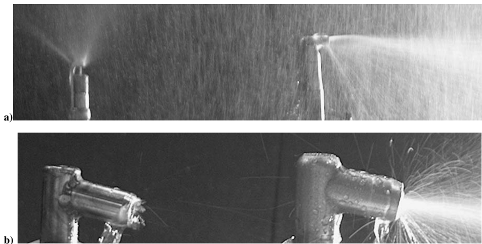
Fig. 7 Spray atomization of existing (left) and modified atomizers (right) (see Fig. 1a and 1c, \beta = 180 deg): a) without vaporizer housing and b) with vaporizer housing; liquid pressure drop 1.5 bar and air velocity 20 m/s.
